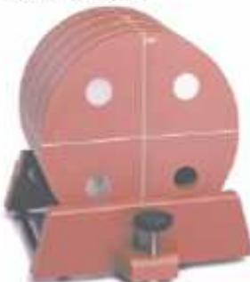
The optional phantom base (shown at left with the phantom) provides stability, marker alignment master and features built-in leveling device.
